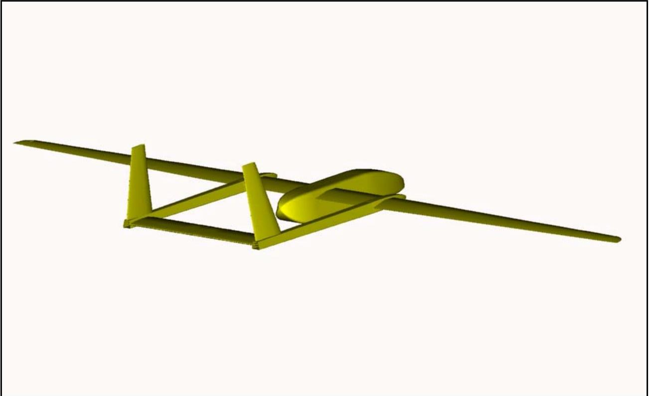
Figure 1 HALE UAV Concept
