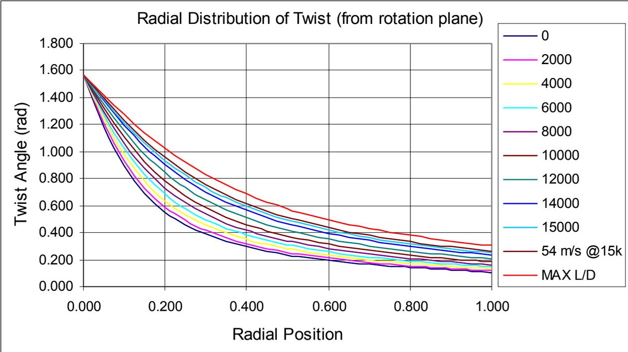
Figure 3 Radial Distribution of Twist for Various Optimal Propellers
