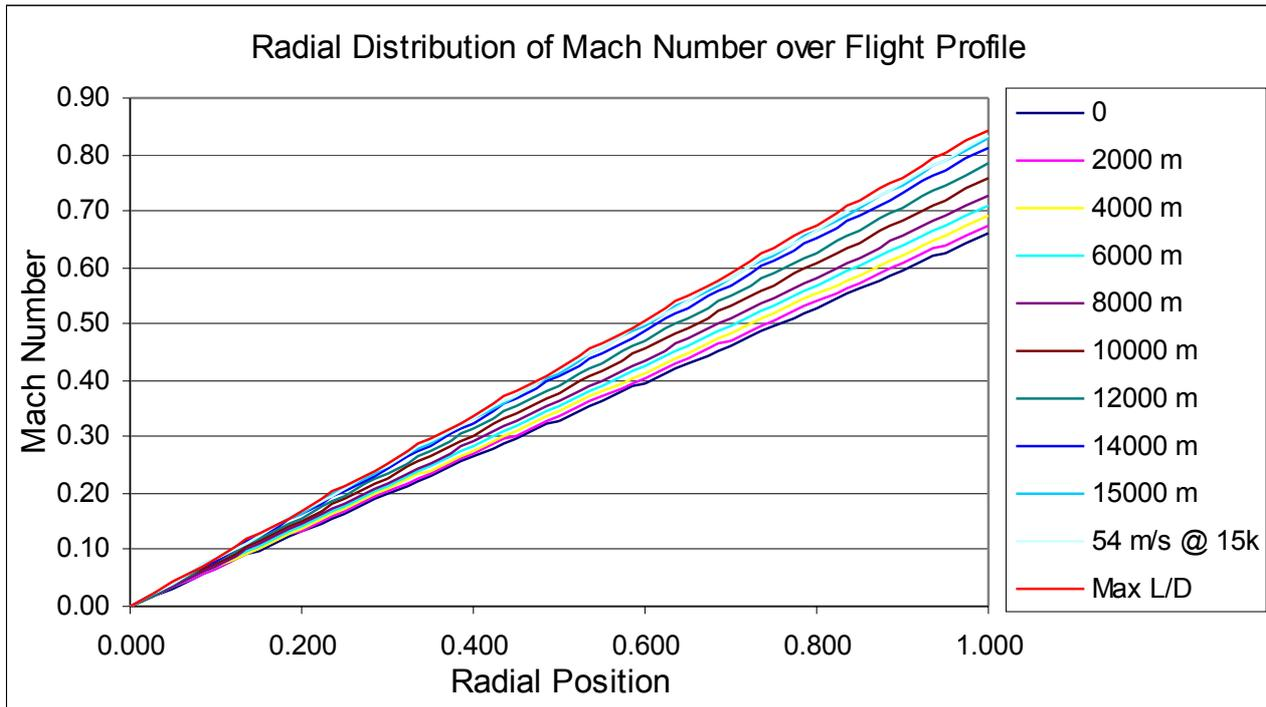
Figure 5. Radial Distribution of Mach Number for Various Optimal Propellers
