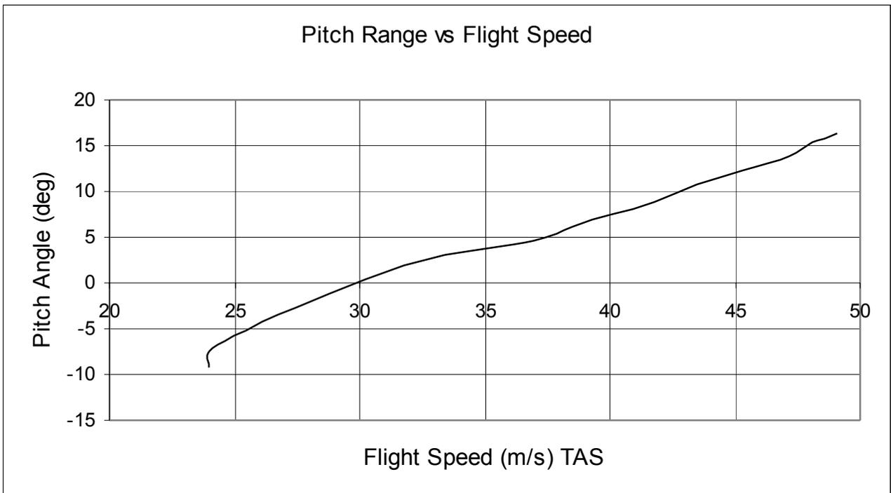
Figure 9. Pitch Angle Variation with Airspeed for Final Propeller
