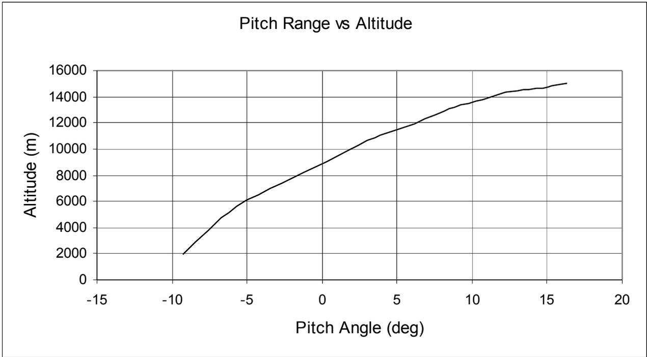
Figure 8. Pitch Angle Variation with Altitude for Final Propeller
