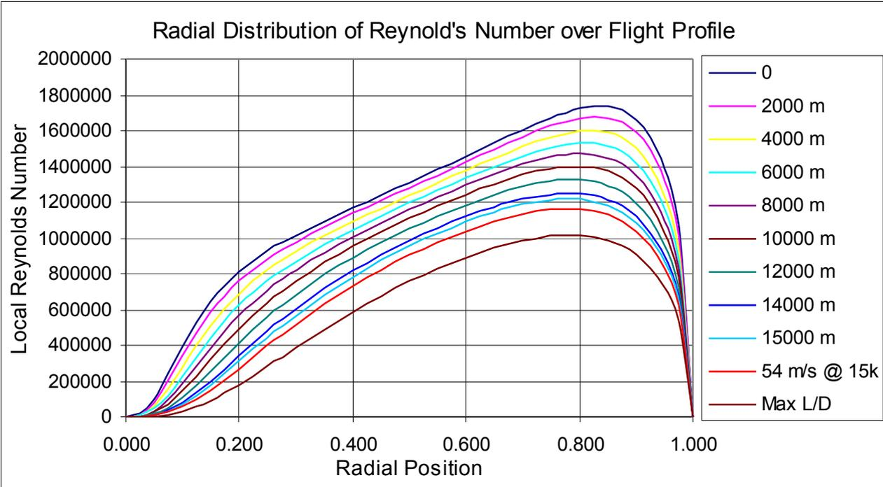
Figure 4 Radial Distribution of Reynolds Number for Various Optimal Propellers
