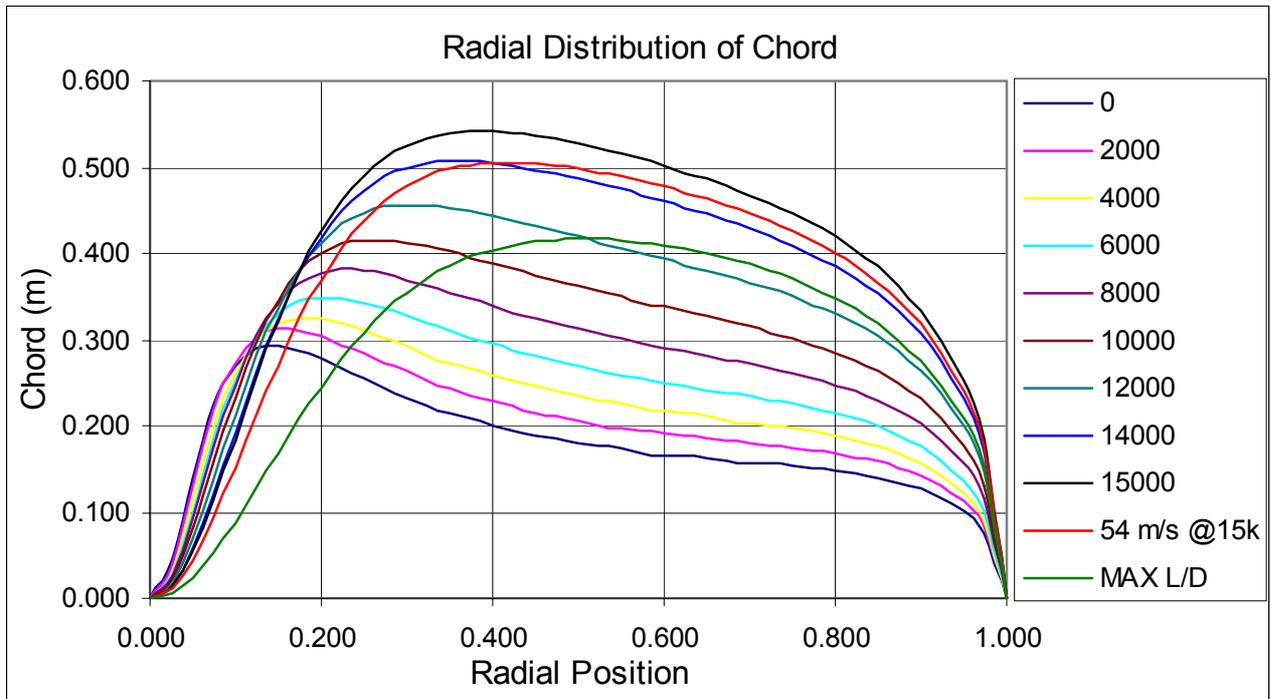
Figure 2. Radial Distribution of Chords for Various Optimal Propellers
