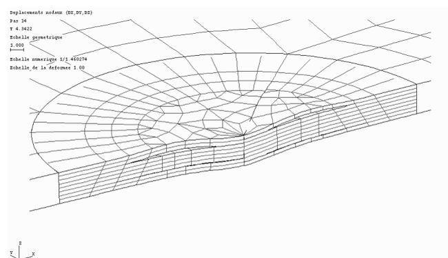
*Fig. 8 - propagating delamination under in-plane compression of the laminate*
