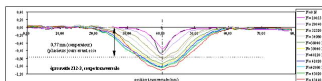
Fig. 3 - measured impact external induced damaged area on a sandwich panel
