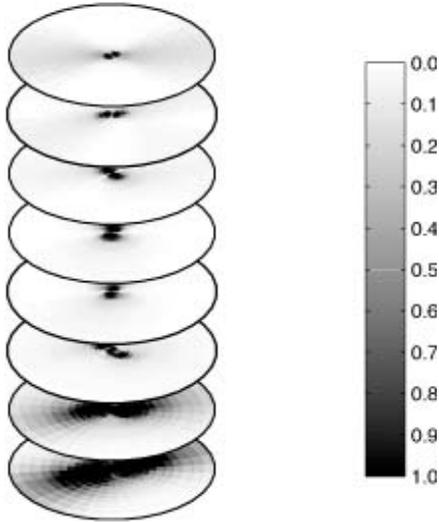
Fig. 6 - damage calculation results in the plies
