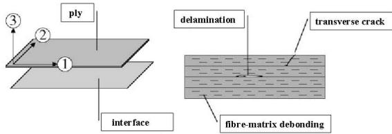
Fig. 4 – damage mesomodel -
