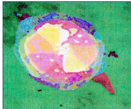
Fig. 1 - US C-Scan of a  $(45^{\circ}_2, 0^{\circ}_2, -45^{\circ}_2, 90^{\circ}_2)_S$ , 7.1 J impacted T300/914 laminate
