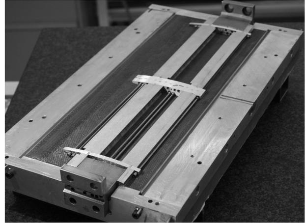
**Fig. 4** Upper shell of the second model with rib, spars and flanges
