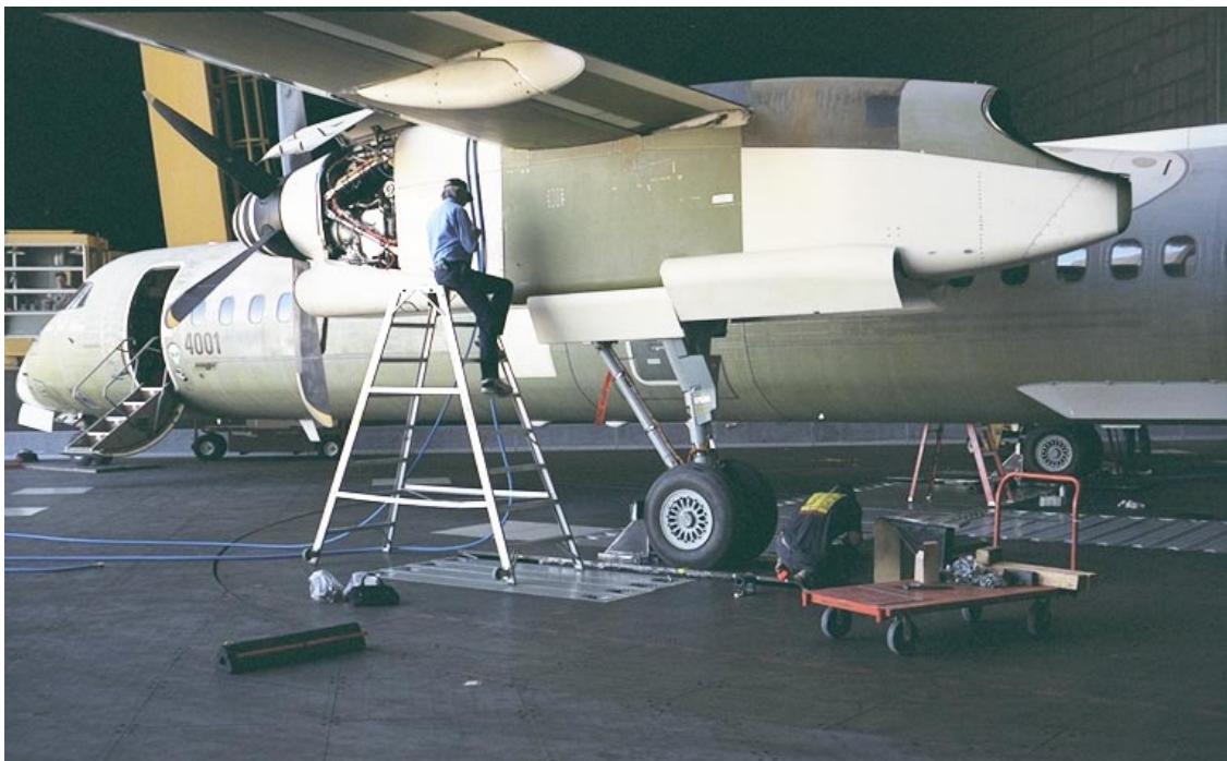
Figure 2 Showing Fuel & Nitrogen Hoses, MLG Restraints & Turntable
