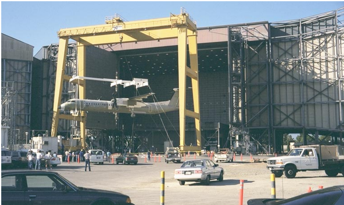
Figure 1 Lifting the Aircraft into the 80x120' Wind Tunnel
