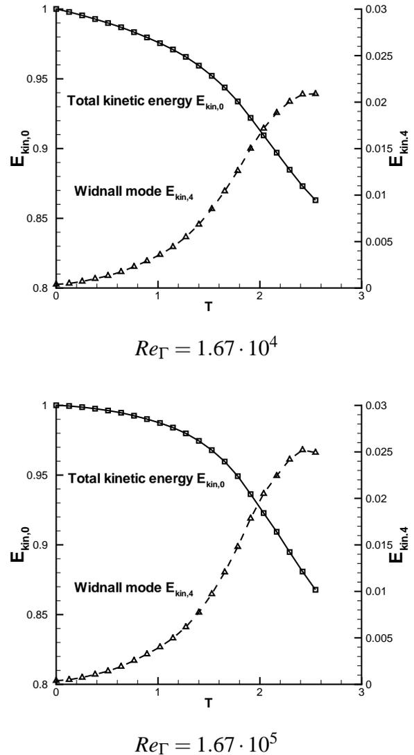
**Fig. 4** Kinetic energy within computational domain: evolution of coefficients of Fast Cosine Transform in axial direction  $k = 0$  (total) and  $k = 4$  (wave number of instability).
