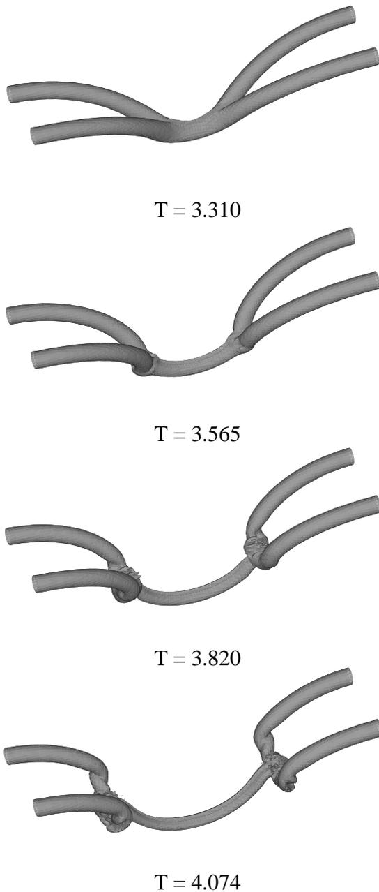
**Fig. 1** Temporal evolution of Crow instability:  $Re_\Gamma = 1.67 \cdot 10^4$ ,  $128^3$  mesh,  $r_c/b = 0.2$ ,  $\lambda/b = 8.0$ . Shown are iso-surfaces  $|\underline{\omega}| = 500 \text{ s}^{-1}$ .
