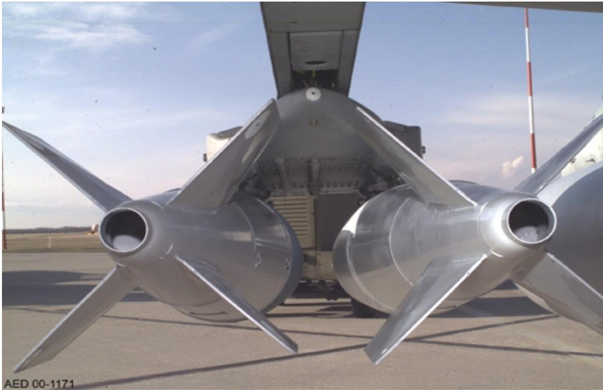
**Figure 9: CF-18/MK-83 Carriage Position**
