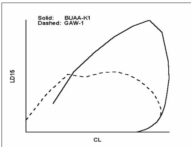
Fig. 4. Comparison of the calculated endurance factor curves
