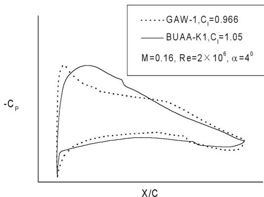
Fig. 1. Target  $C_p$  distribution of the new airfoil and the comparison with that of the GAW-1
