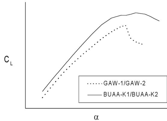
Fig. 8. Comparison of the measured wing/body lift curves
