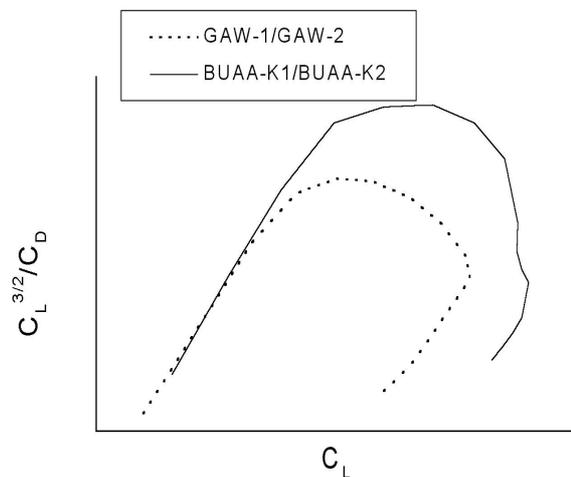
Fig. 9. Comparison of the measured wing/body endurance factor curves
