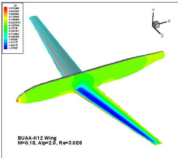
Fig. 7. Calculated surface Cp distribution and isobars of the BUAA-K12 wing/body configuration
