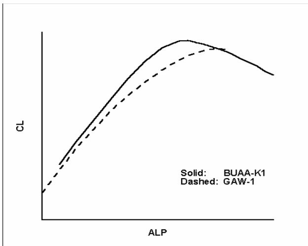
Fig. 3. Comparison of the calculated lift curves
