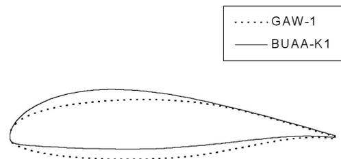
Fig. 2. Contour of the new airfoil BUAA-K1 and the comparison with GAW-1
