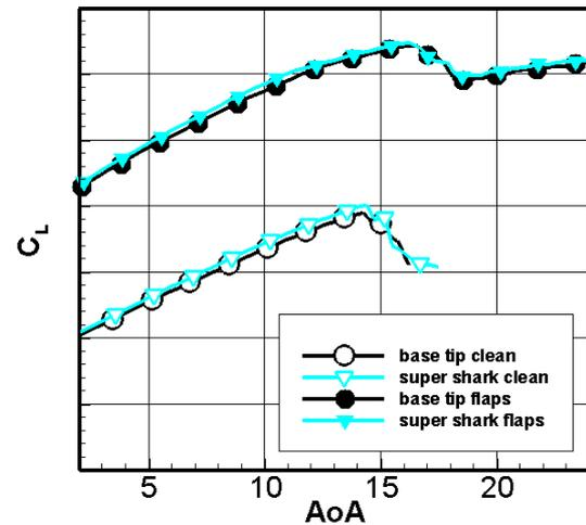
**Fig. 10 lift  $C_L$  incl. maximum lift  $C_{Lmax}$  for clean and full flaps over  $\alpha$  - SuperShark™ and base tip**
