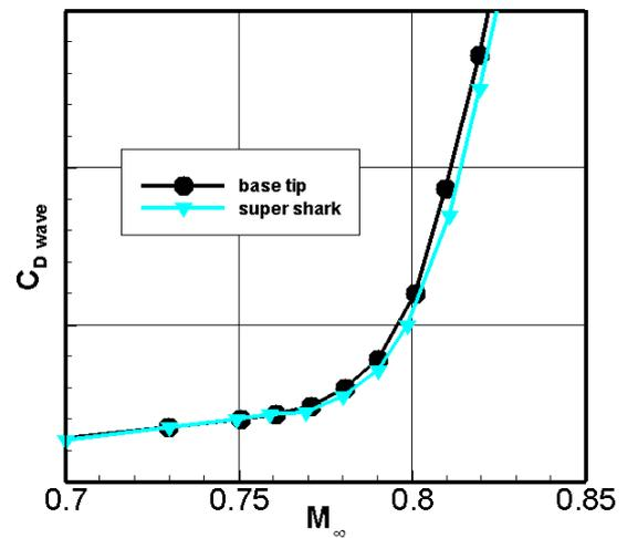
Fig. 13 drag rise – wave drag  $C_{Dwave}$  over Mach number for constant lift coefficient
