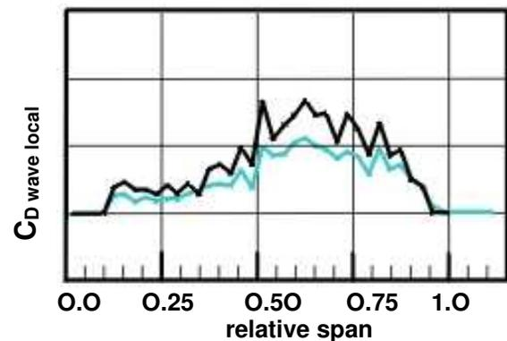
Fig. 14 wave drag  $C_{D wave local}$  along relative wing span with and without SuperShark™
