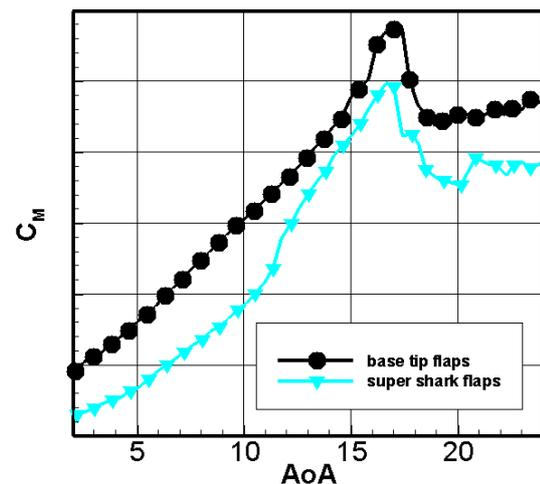
**Fig. 11 pitching moment  $C_M$  over angle of attack  $\alpha$  corresponding to the lift  $C_L$ , fig 10.**
