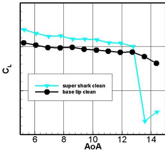
Fig. 12 aileron efficiency – Rolling moment  $C_L$  over angle of attack  $\alpha$  – SuperShark™, base tip
