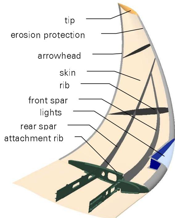
**Fig. 16** structural layout of the SuperShark<sup>TM</sup>
