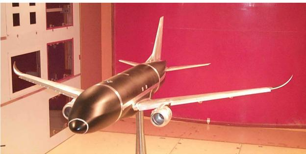
**Fig. 9 low speed model – scale 1:13**
