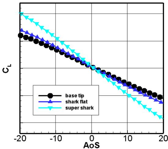
**Fig. 15** roll due to yaw – Rolling moment  $C_L$  over angle of sideslip  $\beta$  for clean aircraft – Shark Flat, SuperShark<sup>TM</sup> and base tip
