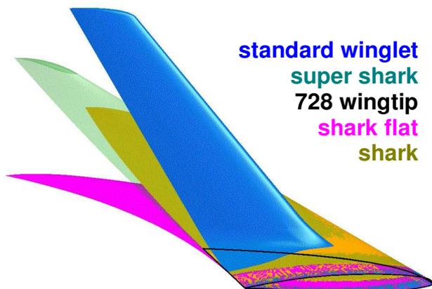
**Fig. 1** perspective view of the baseline wingtip, the standard winglet and the Shark family
