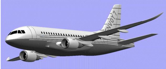
**Fig. 17 corporate jet including a wingtip extension out of the new Shark family**
