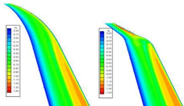
**Fig. 3** isobars on the topview of the SuperShark<sup>TM</sup> and the standard winglet
