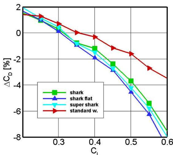
Fig. 6 resulting drag improvement  $\Delta C_D$  over lift  $C_L$
