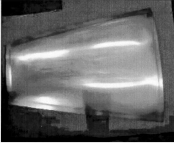
**Figure 20.** Seamless Glare tubes.
