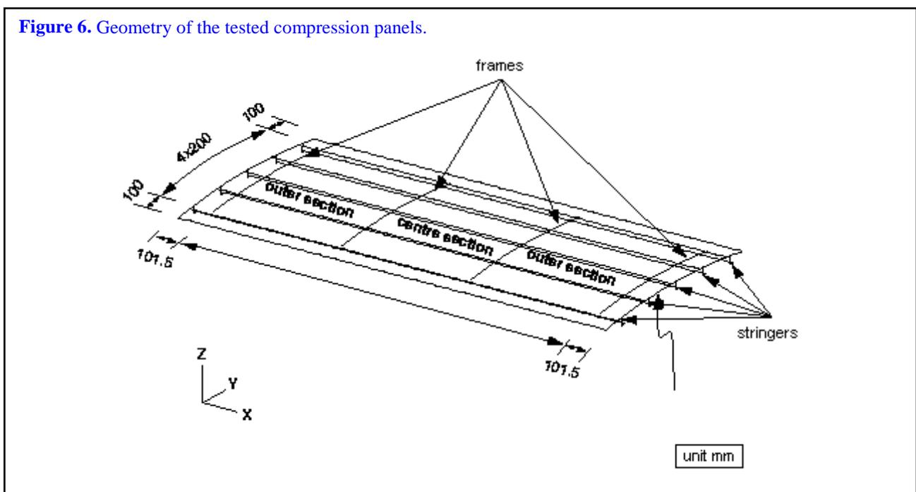
the Euler-Johnson method for compression loading and Kuhn's method for shear loading, were modified and supported by finite element calculations. For compression two panels such as indicated in Fig.6 were designed and tested. Also large (1 x 1 m<sup>2</sup>) shear panels were designed and tested using a picture frame test (see Fig.7). Both the compression and the shear behaviour could be accurately predicted by finite element calculations.
