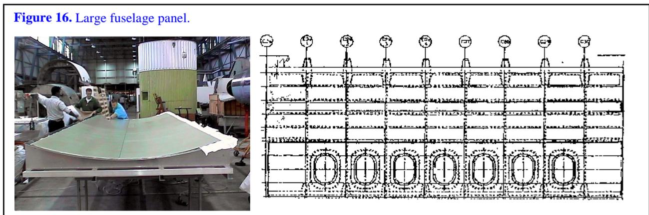
**Figure 16.** Large fuselage panel.
