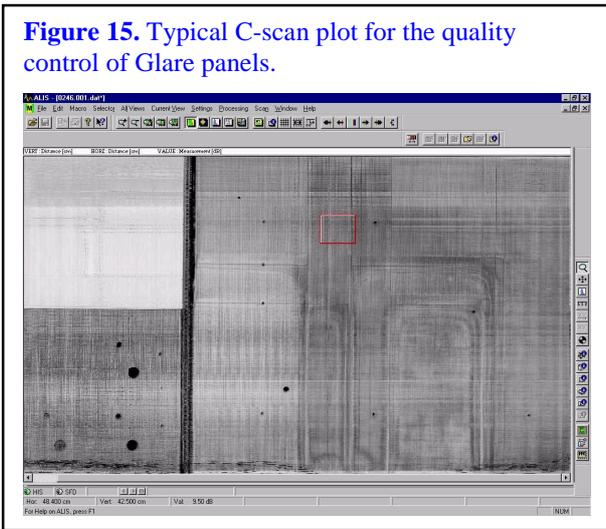
**Figure 15.** Typical C-scan plot for the quality control of Glare panels.
