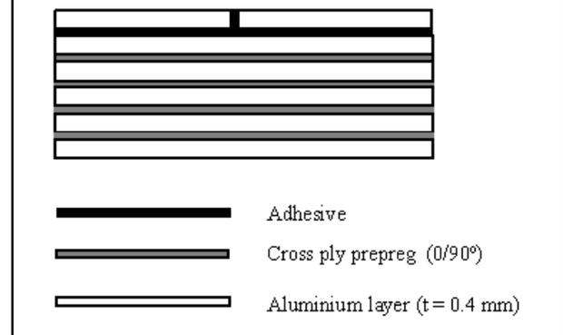
**Figure 6.** Geometry of the tested compression panels.
