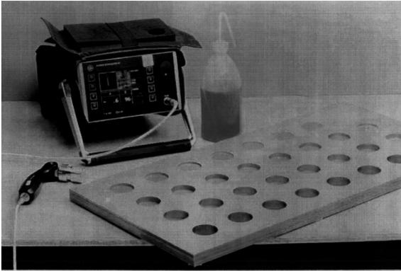
Glare lay-ups with standard inspection techniques. For the detection of surface cracks Eddy Current inspection and Magneto Optic Eddy Current Imaging were studied. Eddy Current inspection also proved suitable for tracing sub-surface cracks in Glare.
