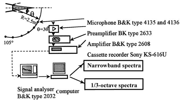
**Fig.1. Scheme of measurement and data processing**
