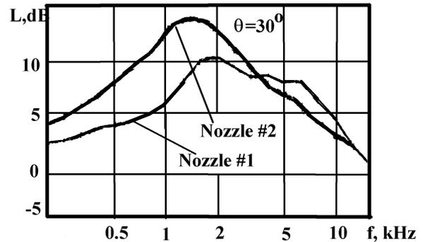
**Fig.4 Efficiency of axisymmetrical ejector nozzle**
