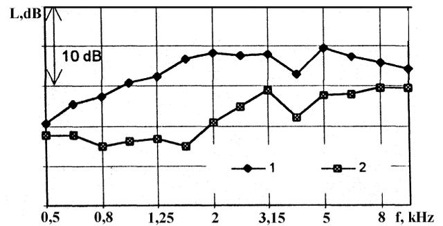
**Fig.9. Comparison of sound pressure levels for treated and non-treated ejectors in the maximum radiation direction**
