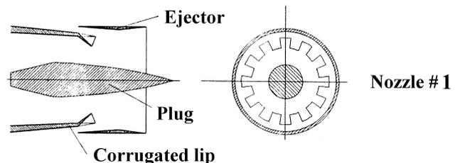
**Fig.2. Scheme of axisymmetrical ejector nozzle**
