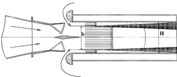
Fig.5. Scheme of flow in ejector duct
