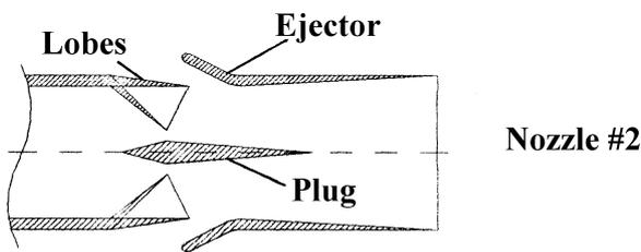
**Fig.3. Scheme of the multi-element ejector nozzle of rectangular shape**
