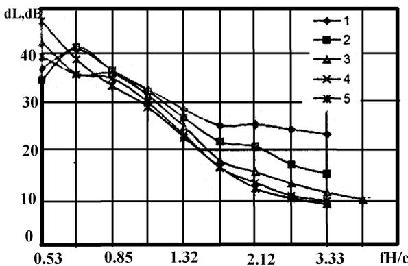
**Fig.6. Frequency dependence of optimum attenuation at different source positions and at unequal opposite wall impedance of plane ejector**
