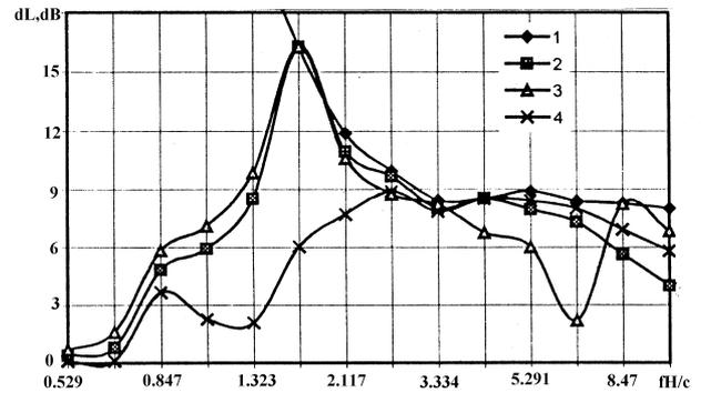
Fig.7. Comparison of attenuation frequency spectra for double-and single-layered treatments with the maximum possible one. 1 – maximum attenuation, 2 – double-layered lining, 3 – single-layered,  $f=1.69$ , 4 – single-layered,  $f=4.23$
