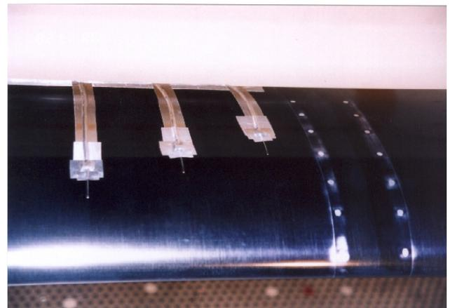
Figure 13 Preston tubes put on the surface
