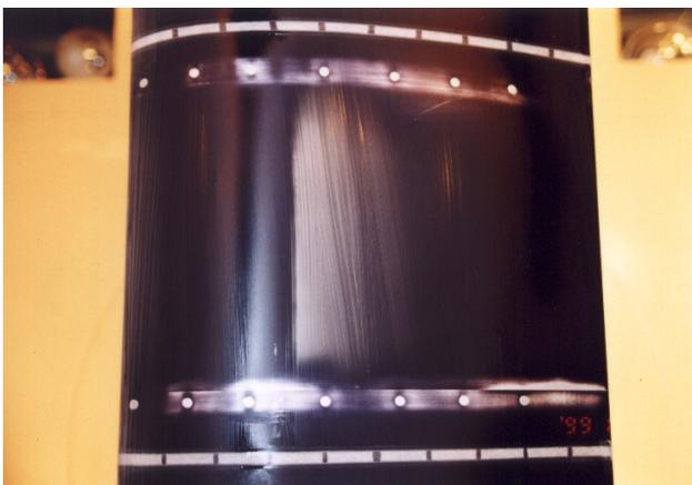
Figure 15 Flow visualization result by China clay technique at  $V=40$  m/s and  $\alpha=10$  degrees
