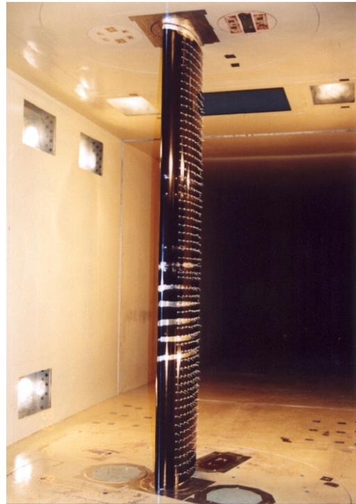
Figure 5 New test model with tufts for flow visualization in NAL gust wind tunnel
