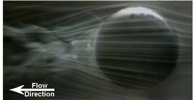
**Figure 5. Smoke filaments over the upper surface at  $10^\circ$  incidence,  $Re = 1.49 \cdot 10^4$ .**
