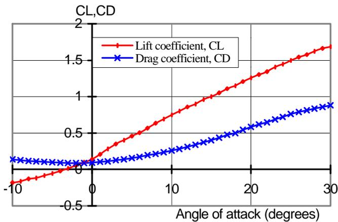
**Figure 2. Lift and Drag characteristics for  $AdvR = 0.46$ ,  $Re = 2.84 \cdot 10^5$ .**
