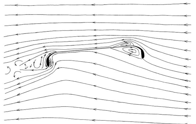
**Figure 5. 2D cross-sectional flow topology for a non-rotating disc-wing,  $5^\circ$  incidence.**
