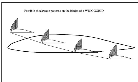
Because the WINGGRID has strictly rectangular lift distribution, it lends itself to a more direct design along the lines of the infinite sheared wing model.
