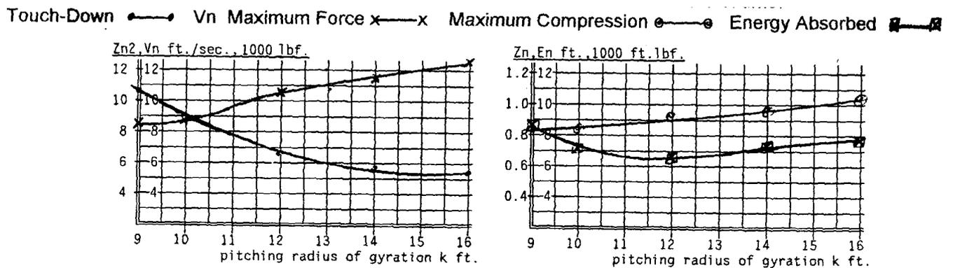
FIGURE 6 a) EFFECT OF AIRCRAFT SCALE ON MOTION, FORCES AND ENERGY ABSORPTION ON MAIN LANDING GEARS at instants of time:
