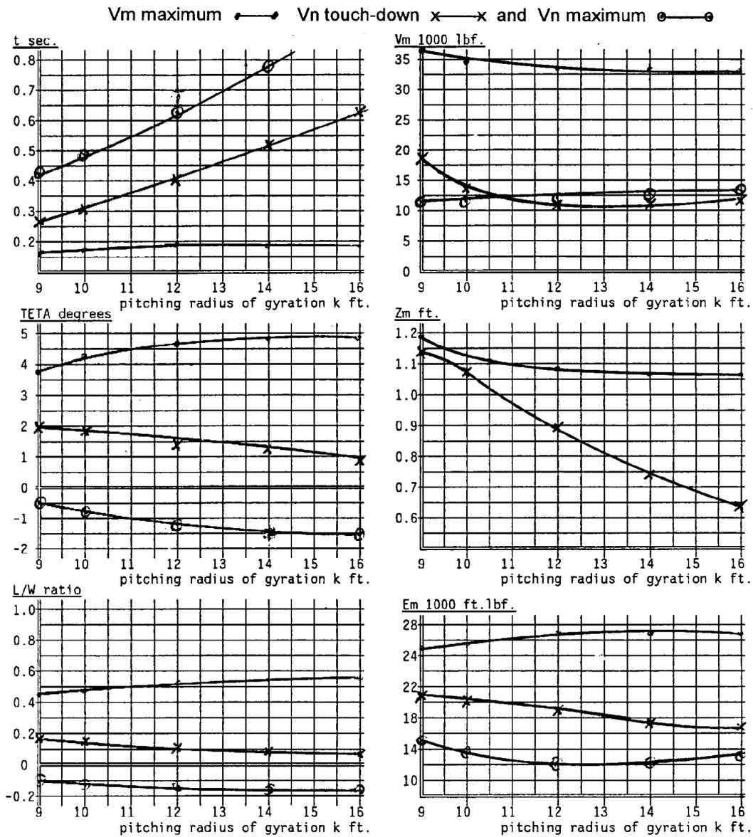
FIGURE 5 b) EFFECT OF PITCHING MOMENT OF INERTIA ON MOTION, FORCES AND ENERGY ABSORPTION ON NOSE LANDING GEARS at instants of time:
