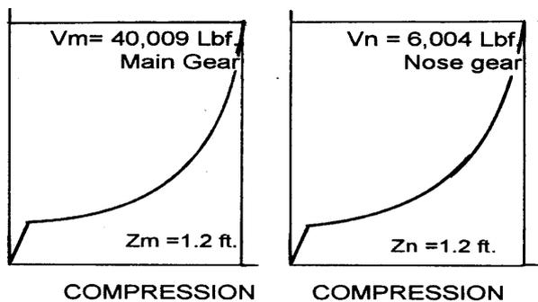
For the nose gear it might be assumed that the loading conditions are directly proportional to those at the main gear when the "static" mass is taken.
