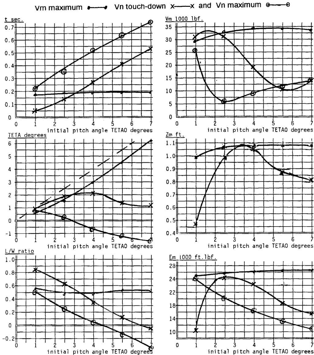
FIGURE 3 b) EFFECT OF INITIAL PITCH ANGLE ON MOTION, FORCES AND ENERGY ABSORPTION ON NOSE LANDING GEARS at instants of time:
