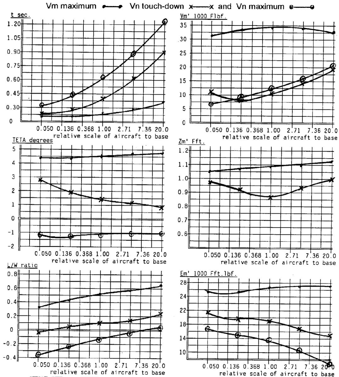
FIGURE 6 b) EFFECT OF AIRCRAFT SCALE ON MOTION, FORCES AND ENERGY ABSORPTION ON NOSE LANDING GEARS at instants of time:
