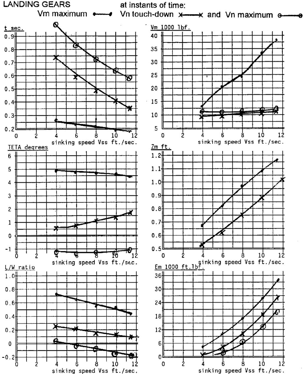
**FIGURE 4 b) EFFECT OF SINKING SPEED ON MOTION, FORCES AND ENERGY ABSORPTION ON NOSE LANDING GEARS**
