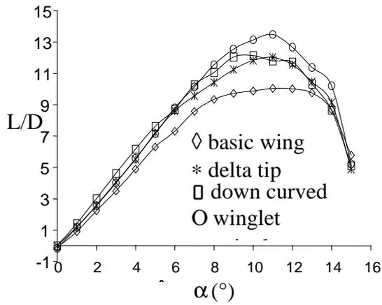
Fig. 5 Effect of wing tip devices on aerodynamic efficiency
