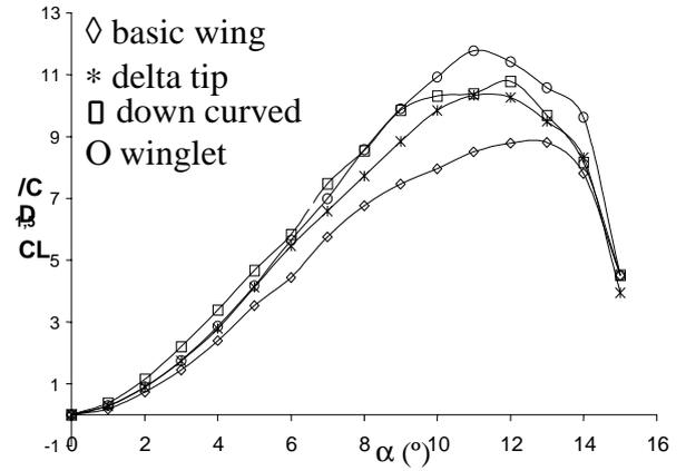
Fig. 6 Effect of wing tip devices on rate of climb factor
