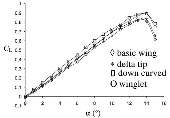
Fig. 2 Effect of wing tip devices on lift coefficient
