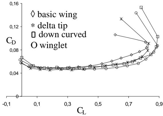
Fig. 4 Effect of wing tip devices on drag polar
