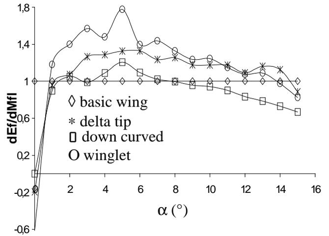
Fig. 7 Effect of wing tip devices on ASEP parameter
