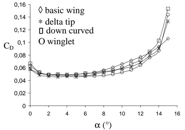
Fig. 3 Effect of wing tip devices on drag coefficients
