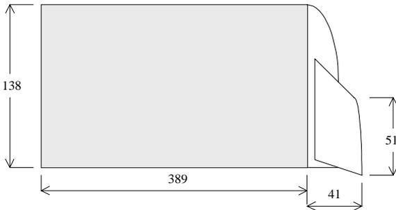
Fig. 1 a),b),c). Wing tip configurations studied (dimensions are in millimeters)
