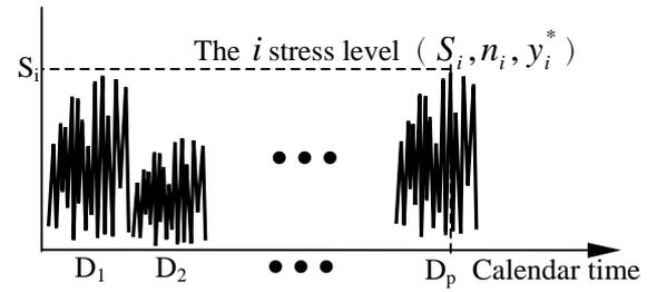
Fig.5: Calendar loading spectrum of aircraft
