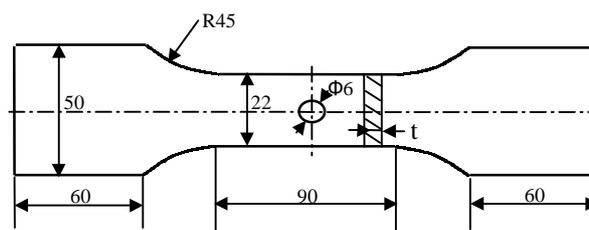
Fig.1: The central-hole specimen (for LC4CS t=4, for 30CrMnSiNi2A t=7; dimension in mm)
