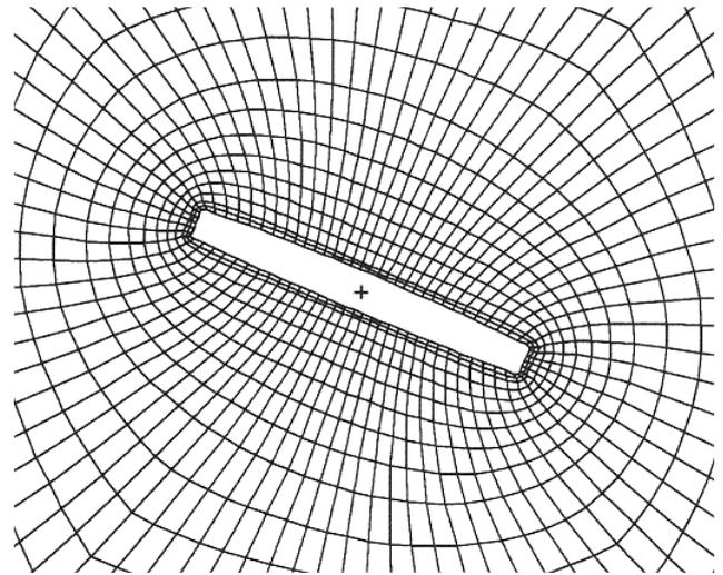
Figure 11 Optimum cut-out under 1:2 shear/compression loading for an isotropic plate
