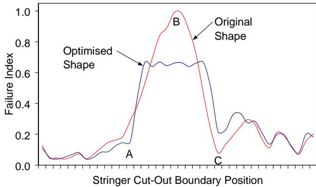
Figure 14 Variation in failure index around the stringer cut-out boundary for the original and optimised shapes
