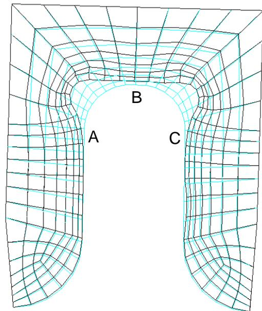
Figure 13 Optimised stringer cut-out shape (original shape shown in light blue)
