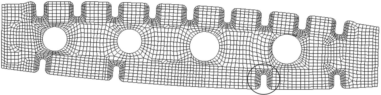
Figure 12 Full rib model (critical stringer cut-out circled)
