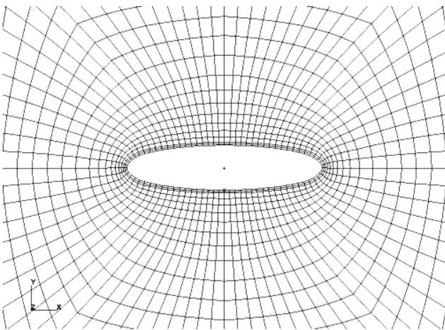
**Figure 5 Optimum cut-out under 4:1 uniform bi-axial load for Laminate 1**
