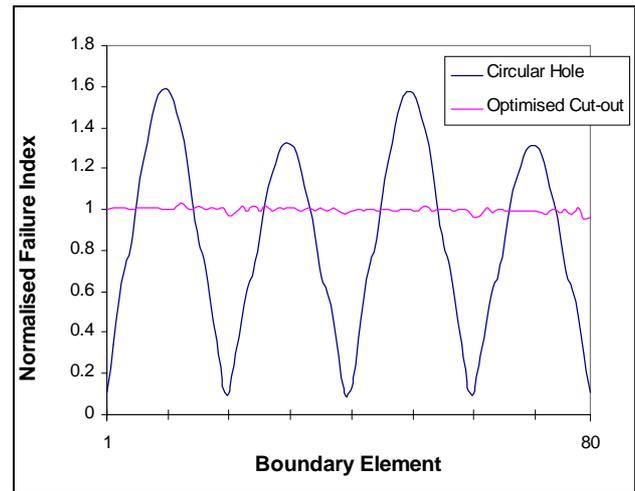
**Figure 8 Normalised boundary failure indices for Laminate 1 under shear load**
