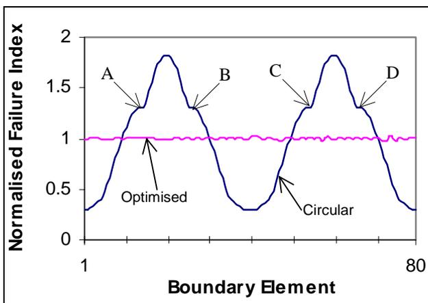
**Figure 6 Normalised boundary failure indices for Laminate 1 under 2:1 bi-axial load**
