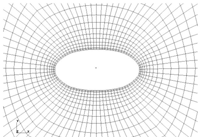
**Figure 4 Optimum cut-out under 2:1 uniform bi-axial load for Laminate 1**
