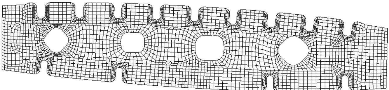
Figure 15 Rib model showing optimised access holes
