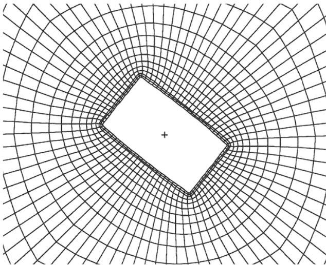
Figure 9 Optimum cut-out under 1:0.5 shear/compression loading for an isotropic plate
