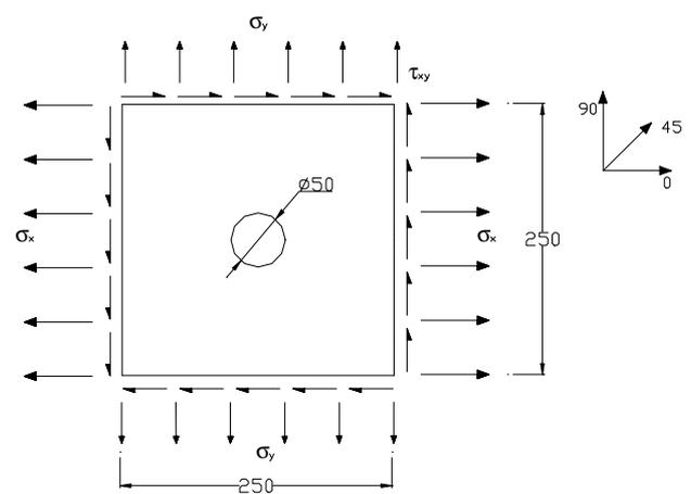
Figure 1 Square plate with central hole (in mm)
