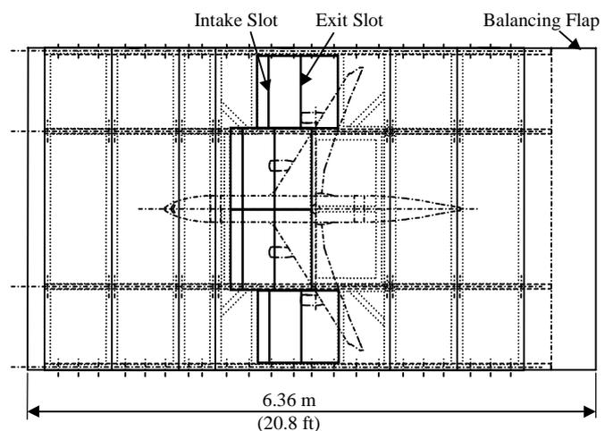
Figure 3. Plan view of the ground plane showing the BLCU positions and A340 model
