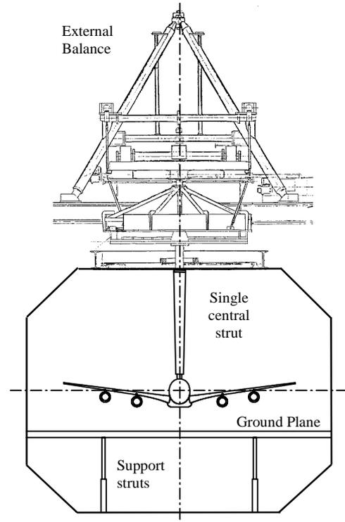
Figure 2. Ground effect testing arrangement
