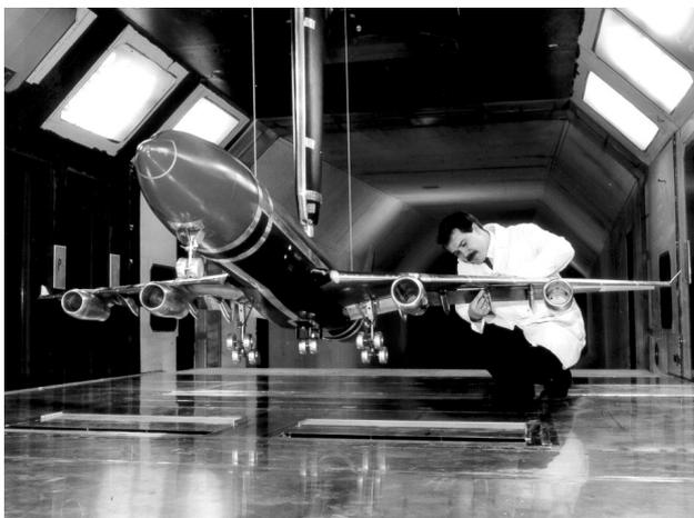
Figure 7 An early A340 ground effect test using two BLCUs
