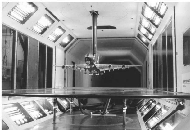
**Figure 10** The A3XX model in the Filton Low Speed Wind Tunnel above the ground plane
