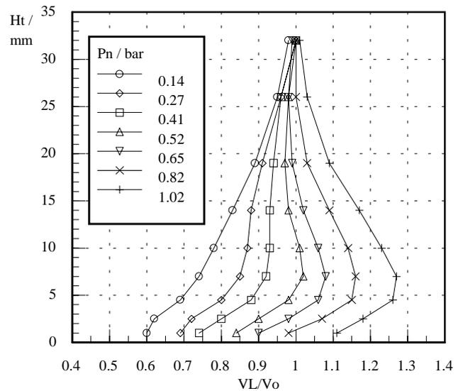
Figure 5 Boundary layer profile sequence as primary nozzle pressure is increased
