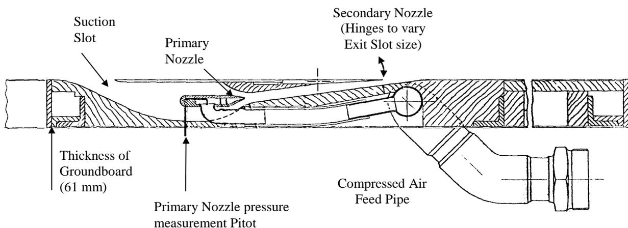
Figure 4 Section through a Boundary Layer Control
