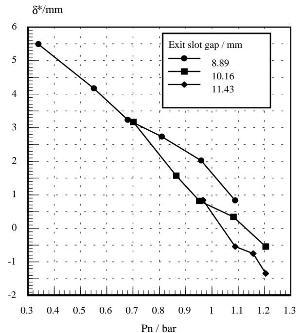
Figure 6. Effect of increasing the exit slot gap
