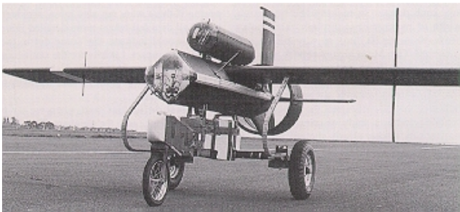
Figure 1 The MACHAN with initial tricycle launch trolley
