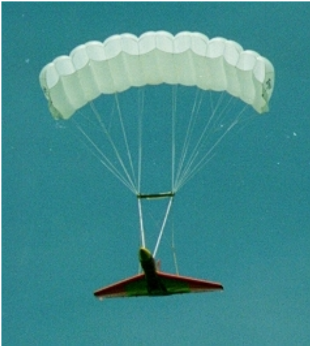
Figure 3 Parafoil recovery of the TTL BANSHEE
