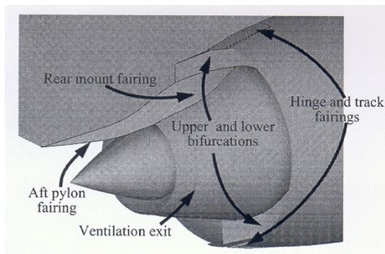
Figure 7: Nozzle and reverser fairings
