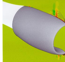
Figure 17: Isolated nacelle shock wave
