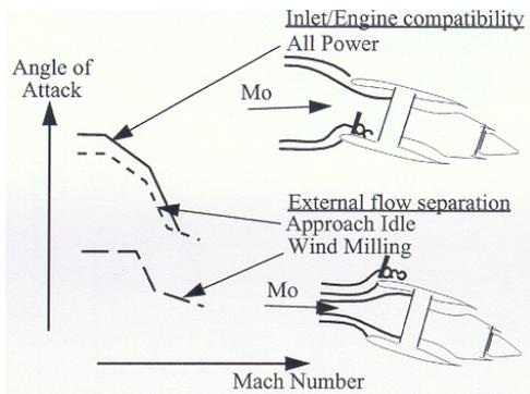
Figure 3: Low speed / high incidence aerodynamic requirements
