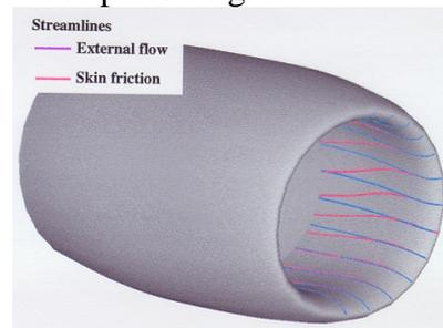
Figure 24: CFD in crosswind conditions
