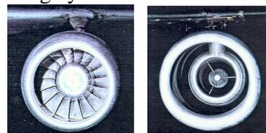
Figure 14: TPS and TFN triple body nacelles
