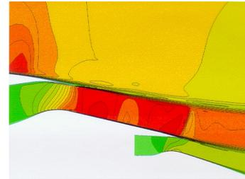
Figure 27: Mach number in the nozzle (Navier-Stokes)
