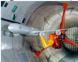
Figure 12: Full span model of aircraft
