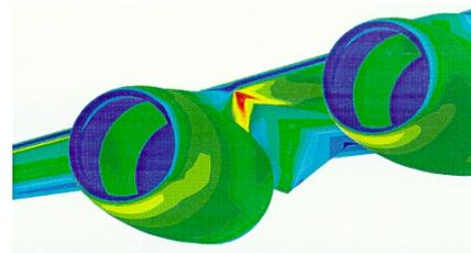
Figure 19: High Mach / Low CL Euler computation of over-speed.
