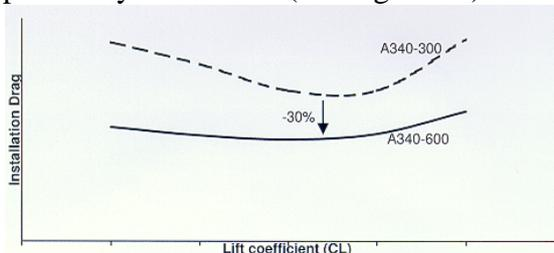
Figure 30: Installation drag of A340-300 and A340-600
