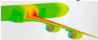
Figure 15: Euler results on complete aircraft
