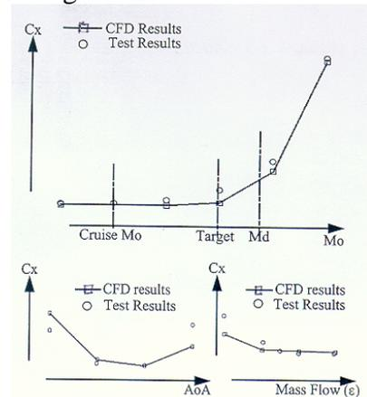
Figure 18: S1 isolated inlet drag results
