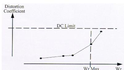
Figure 22: Inlet / Engine compatibility
