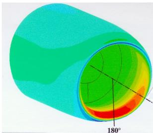
Figure 21: Local Mach number High incidence, high mass flow
