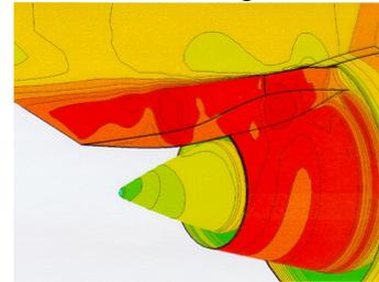
Figure 28: Euler results on 3D nozzle shapes
