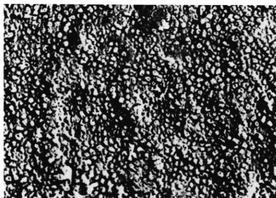
Fig. 13: Phenolic resin replica of a SAA surface 2024 clad
