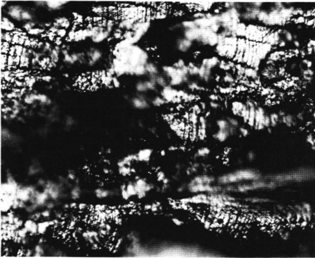
Fig 13. Flight-by-flight striations on the fracture surface of a wing joint of a commercial service aircraft X500.
