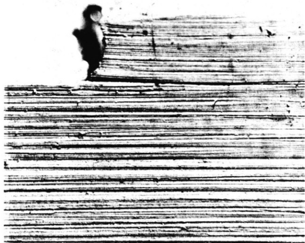
Fig 7. The surface of undercarriage A at the fatigue crack origin showing coarse machining. X100.
