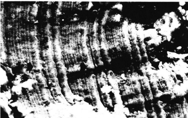
Fig 2. Fatigue striations formed by a complex loading programme used to test military aircraft undercarriages. The crack extension per flight is indicated. X1000.
