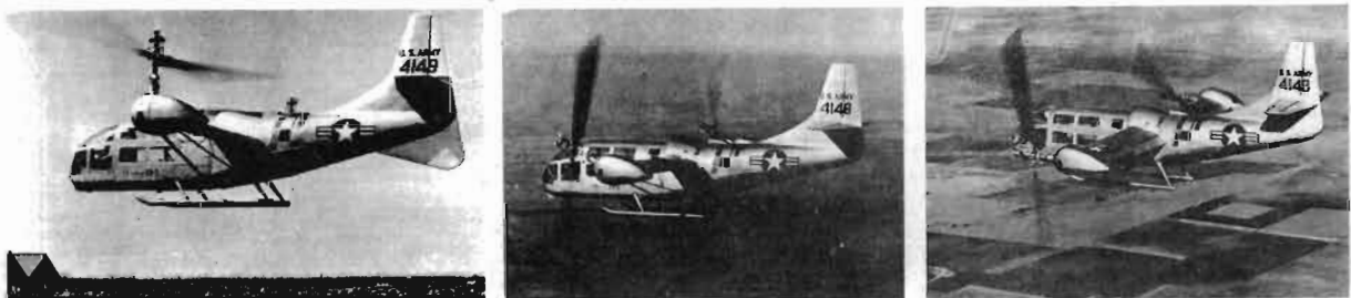
FIGURE 18. BELL XV-3 IN HOVERING, CONVERTING AND CRUISING FLIGHT
