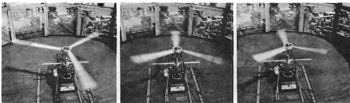
FIGURE 15. VARIABLE-DIAMETER ROTOR TEST SHOWING CONTRACTION TO 60% DIAMETER
