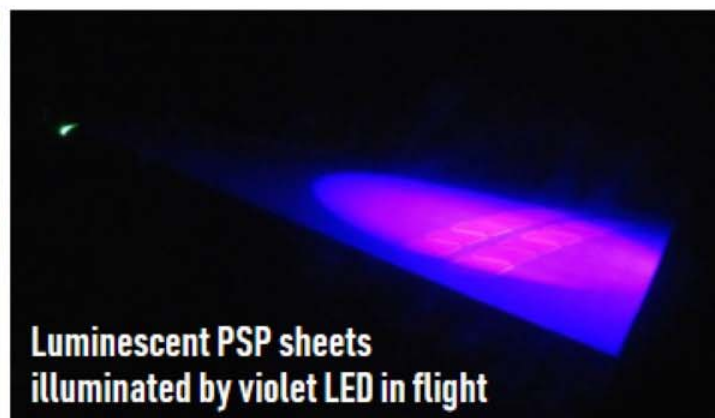
Visualization of shock wave location by in-flight PSP
