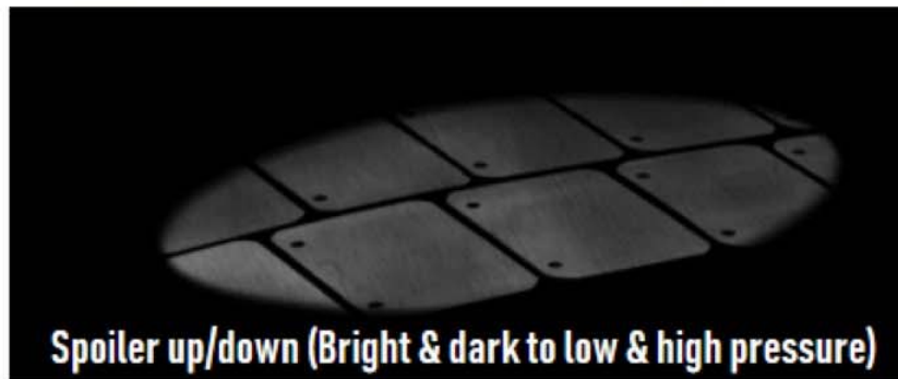
Visualization of shock wave location by in-flight PSP
