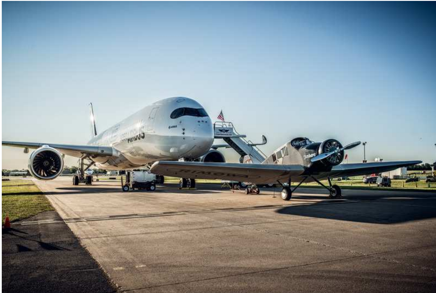
A350XWB (1 st European composite A/C) with Junkers F13 (1 st world all-metal commercial A/C - 1919) – WISCONSIN (USA)
