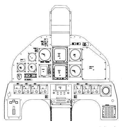
Figure 2: Panel layout of a Pilatus primary Trainer aircraft equipped with a HUD
