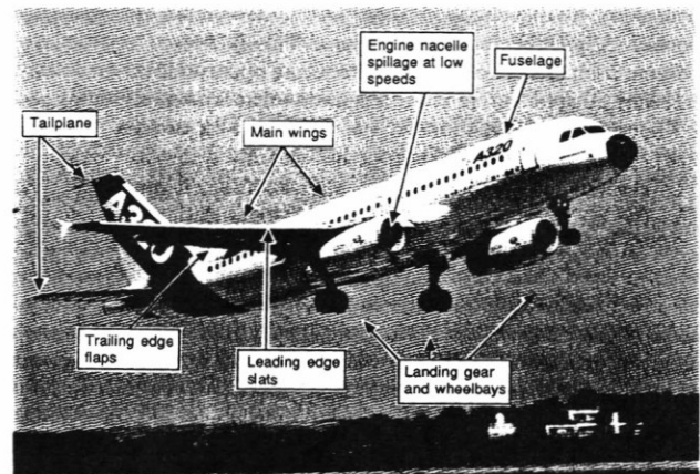
Figure 6. Airframe Noise Sources
