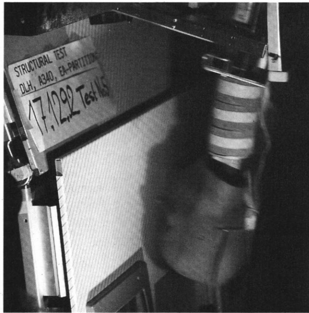
Fig 4 Just before impact, the steel cable which prestresses the neck is completely loosened, the discs between head and pendulum therefore disconnect. Head impact velocity is 15 m/sec.
