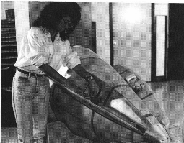
Fig. 12. Installing the pressure transducers in the strakes.
