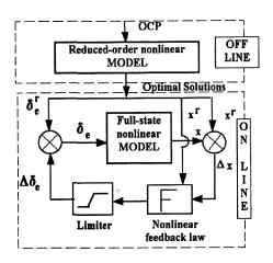
Fig.1 Block diagram schematic of the simulated feedback system
