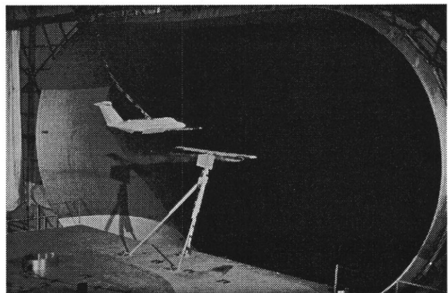
Figure 8. - Free-flight model vortex encounter test.
