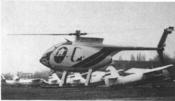
Fig.7 Test helicopter MD Hughes 500 with telemetric system mounted on top of the rotor hub.
