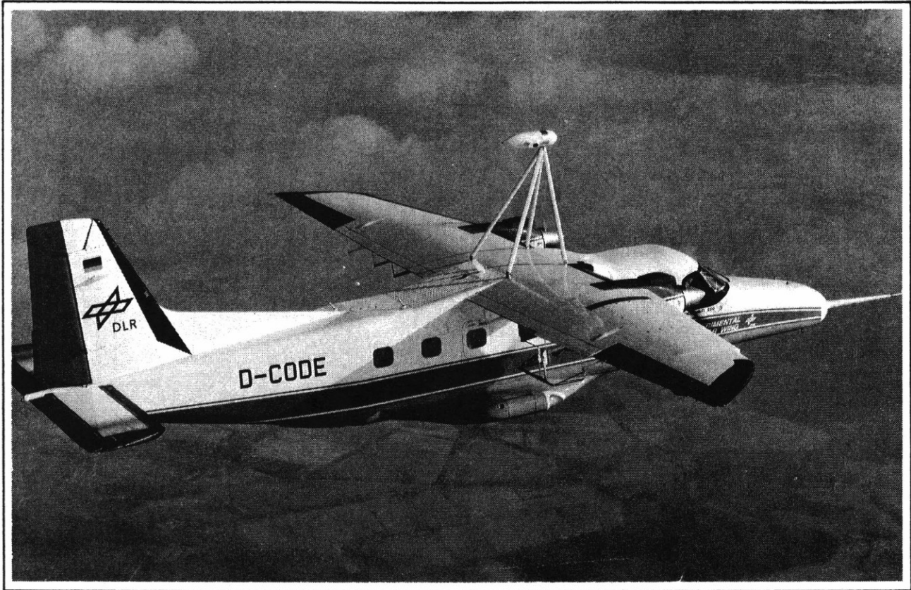
Fig. 1 Do 228 test aircraft with right wing laminar glove
