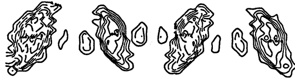
Figure 3(b): Streamwise vorticity contours, M_c=0.4
