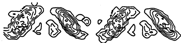
Figure 4(b): Streamwise vorticity contours, M_c=0.8
