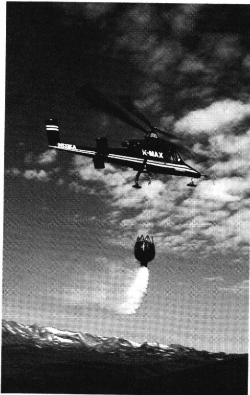
Figure 6. K-MAX ® Lifting Water Bucket.
