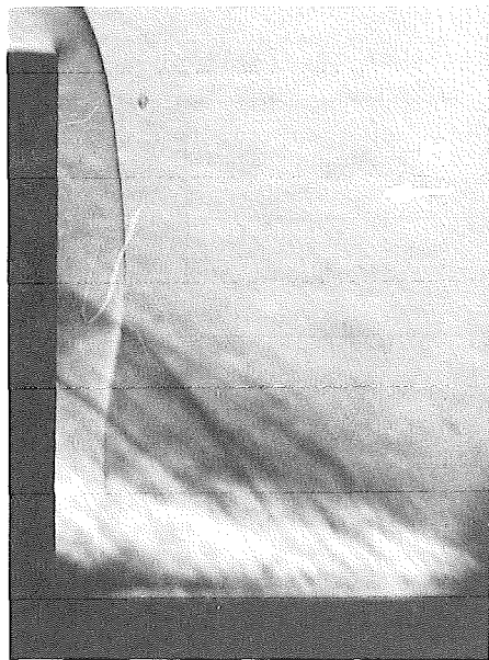
Fig. 4 Horizontal schlieren image for the unswept fin without fillet
