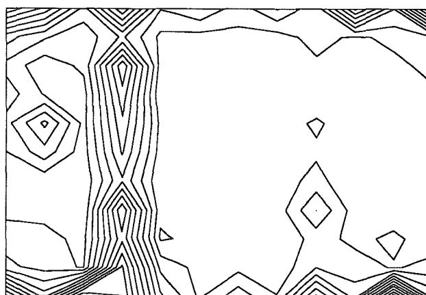
Figure 7 Iso-contours of (a) streamwise turbulence intensity (in percent of freestream velocity, U=25 m/s), Contours start at 0.010 %, increment 0.005 %, (b) vertical turbulence intensity . Contours start at 0.015 %, increment is 0.005 %. Region showed extends from (y,z)=(120,160) mm to (y,z)=(720,1040) mm.
