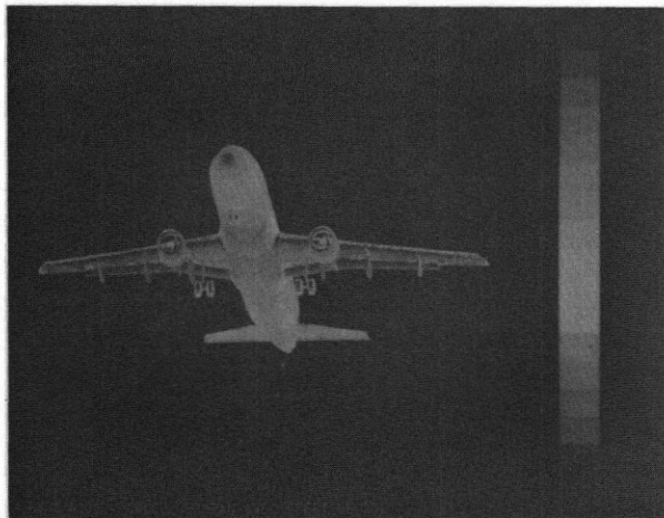
Fig. 26. Airbus front view with wake representation used for the computation.
