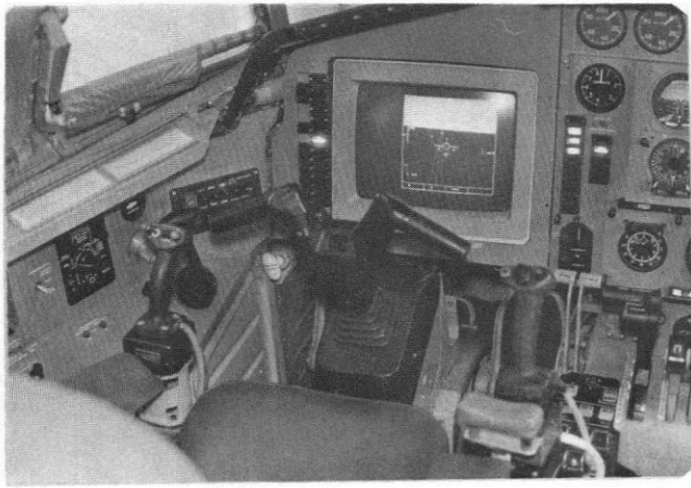
Fig.4. THE LEFT EXPERIMENTAL SEAT OF THE Tu-154M IN-FLIGHT SIMULATOR
