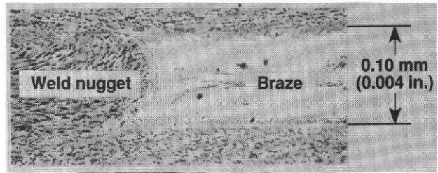
Figure 12. - Weld nugget - braze interface in a weldbrazed titanium skin-stiffener panel.
