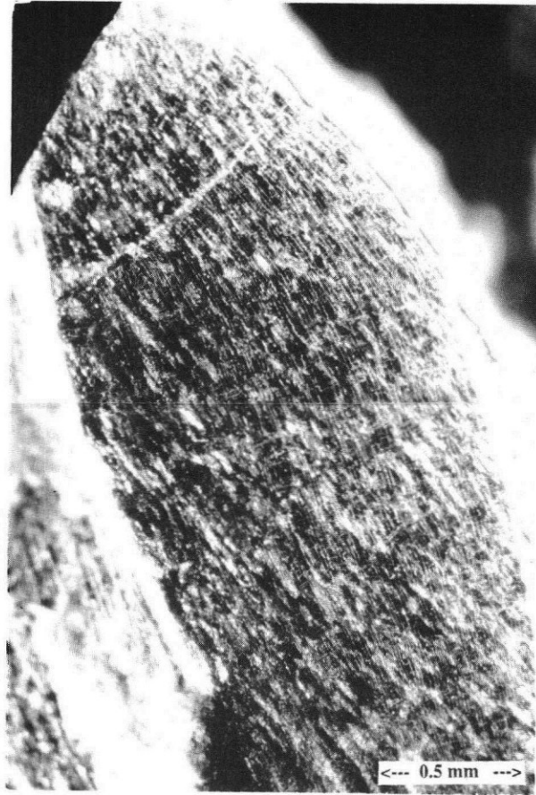
Figure 20. Crack surface of flaw No 3
