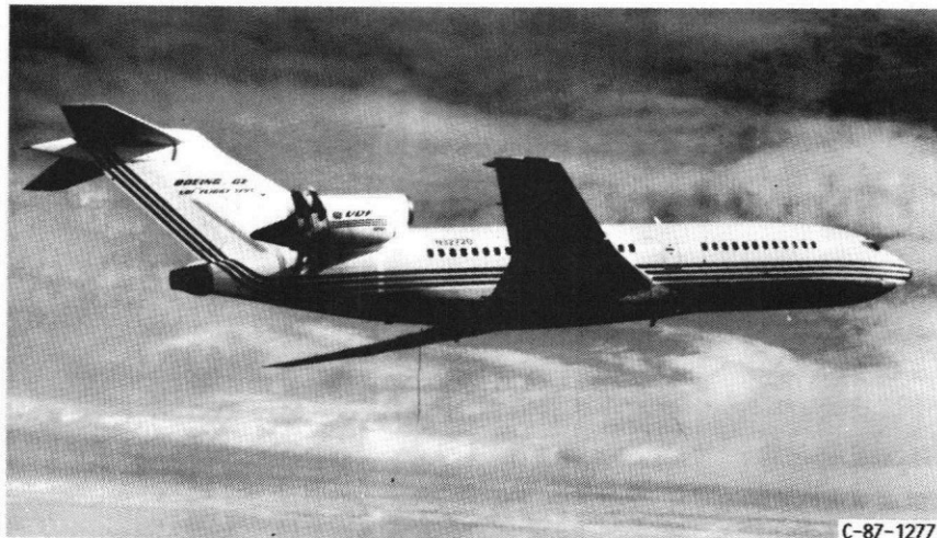
FIGURE 22. - UNDUCTED FAN (UDF) ENGINE ON THE 727 AIRCRAFT.
