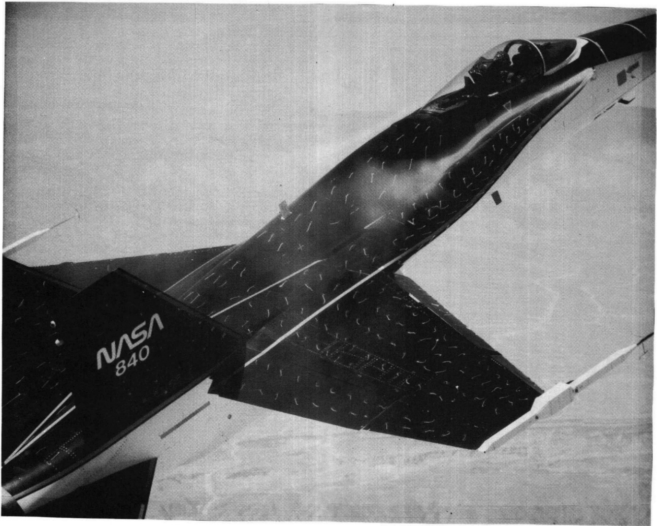
Fig. 18. Flight test surface flow pattern and smoke-flow vortex visualization; \alpha = 30^\circ (Ref. 31).
