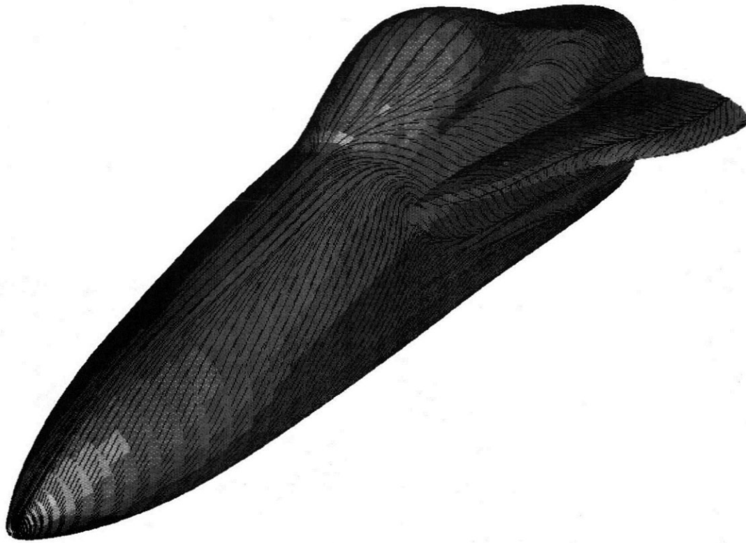
Fig. 6. Fuselage forebody predicted surface flow pattern; M_\infty = 0.2 , \alpha = 19^\circ , Re_\xi = 11.52 \times 10^6 .
