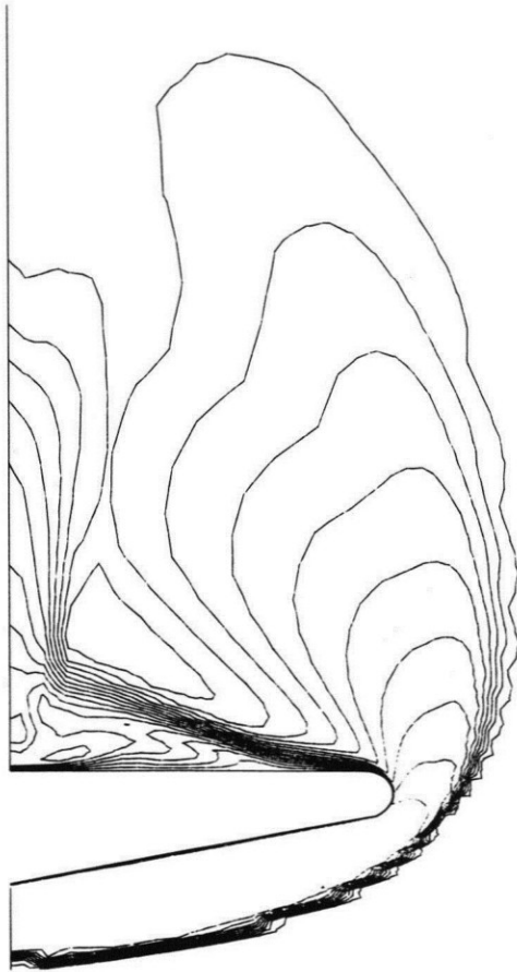
Fig.6. Mach contours at 80% crossflow plane
