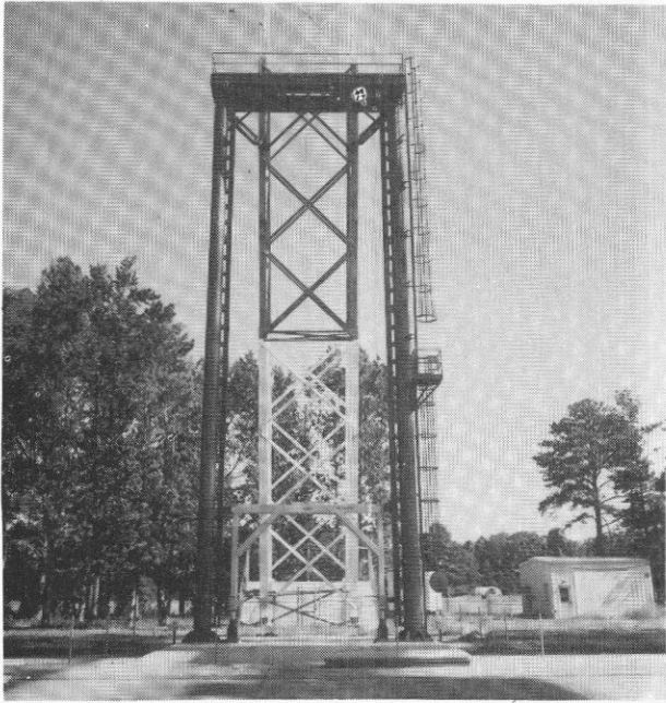
Figure 3. - Vertical Drop Test Apparatus used in testing of aircraft sections and components.
