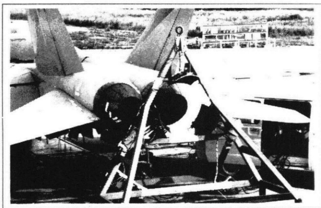
Figure 9. Full Scale Thrust Vectoring System Test Setup
