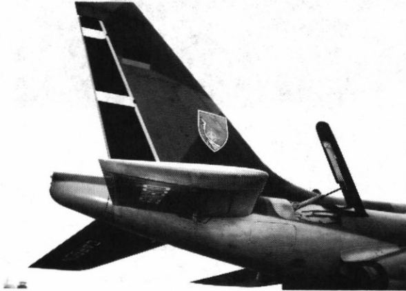
3a) Composite components of the Alpha Jet
