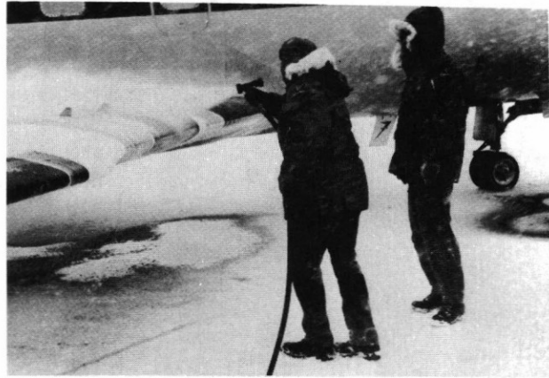
Figure 27 - Ground De-icing of Test Article
