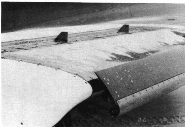
Figure 26 - Extended Krueger With Snow Deposits
