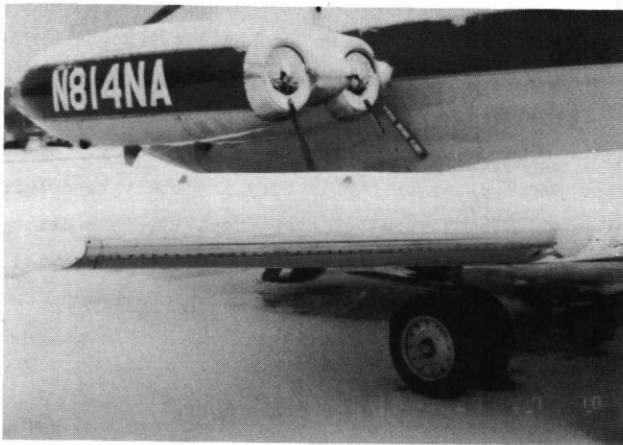
Figure 25 - Snow Deposits on Right Wing
