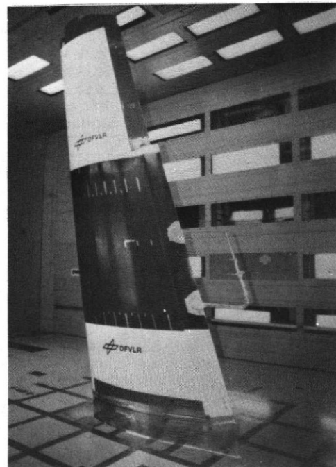
Fig. 11 LFU-205 Wing in the 6x8 m 2 Test Section of DNW
