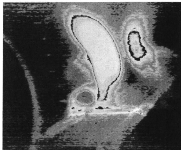
Fig. 4: Nearly concentric brightness pattern of the vortex area visualized by an image processing system.
